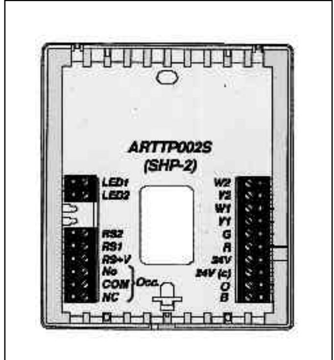
⚡ Jumper between 24V and R must be installed.
