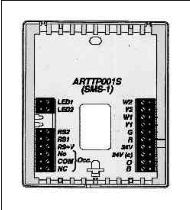
⚡ Jumper between 24V and R must be installed.
